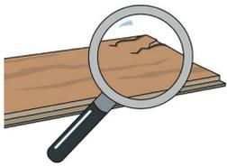
Check all planks for visible defects in optimal light conditions, both before and during installation. Planks with defects must not be used.
