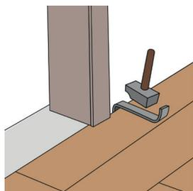
The long sides of the planks have the DuoLoc system. This means the planks can be snapped on the long side using an installation iron, in situations where it is not possible to lift the plank to lock it on the long side.
