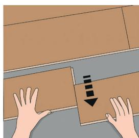
If you want to unlock the 5G loc system, unlock the long side first and then slide the plank towards you without lifting it.
