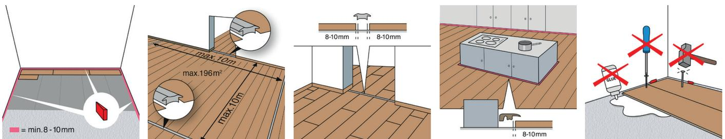
CELLO XXL laminate should be installed as floating flooring which means that the floor should be able to move:
