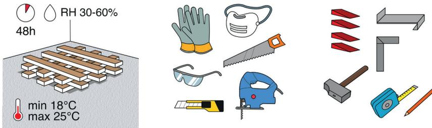
It is important to store the laminate boxes at room temperature for at least 48 hours before the installation. Do not open the packs and stack them in a way so they have maximum contact with the air. The floor should be installed at a room temperature of 18-25°C and a relative humidity of 30-60%
