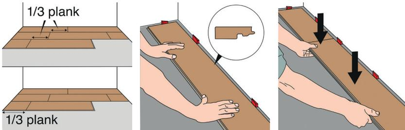
For the most natural floor pattern, make sure to mix the designs of the planks across the floor. The end joints should be staggered min. 1/3 of a plank when installing the floorboards.
