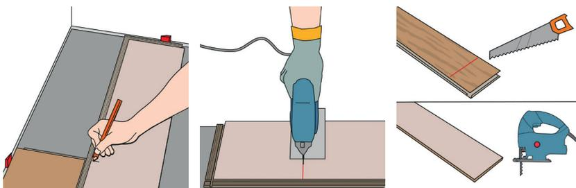
If using a hand saw, cut on the pattern side, if using an electrical jigsaw, always cut on the back side of the plank. A sharp saw blade is a must for the best result!
