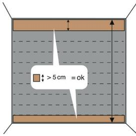
Direction of the planks: the floor will look at its best if installed parallel to the incoming light (short side facing the light).
