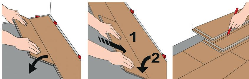
The 5G loc system is extremely easy and fast, it allows you to install large planks with almost no effort. After you have installed the first row, in the second row all you have to do is lock the long side first, and then drop the plank into place on the short side, it will automatically lock.
