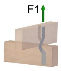
2 Purlin Anchor twist 280 pr. connection
