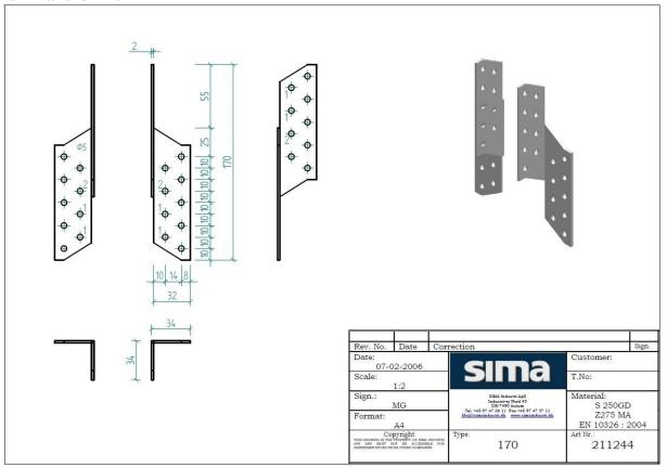
Additionally the bracket can be made from 1,5 mm pre-galvanized steel grades S350GD to Grade S500GD  $\pm$  min. Z275 according to EN 10346 named Purlin Anchor 170PL
