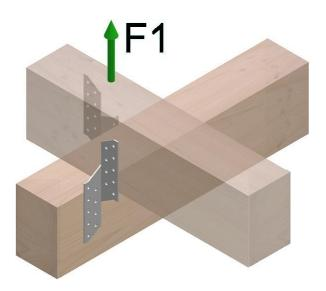
2 Purlin Anchors or Purlin Anchors PL pr. connection in any length
