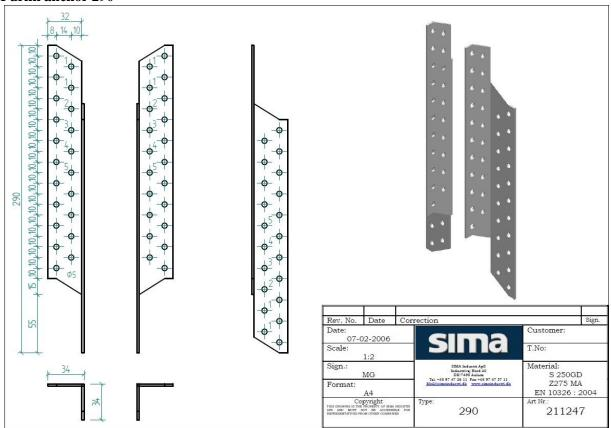
Additionally the bracket can be made from 1,5 mm pre-galvanized steel grades S350GD to Grade S500GD  $\pm$  min. Z275 according to EN 10346 named Purlin Anchor 290PL
