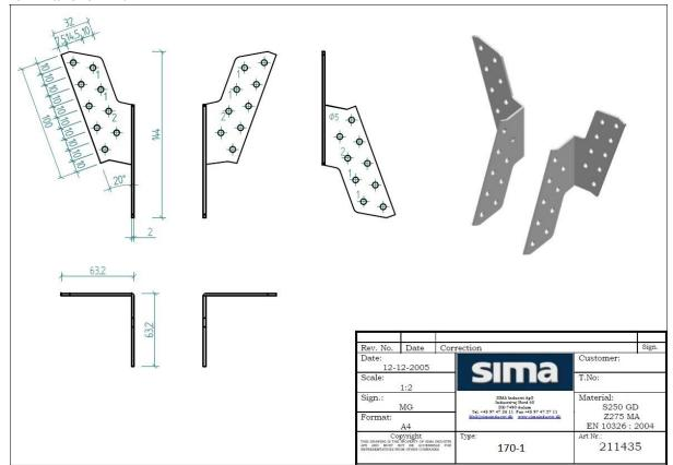
Additionally the bracket can be made from 1,5 mm pre-galvanized steel grades S350GD to Grade S500GD + min. Z275 according to EN 10346 named Purlin Anchor 170-1PL
