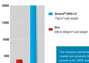
The corrosion performance of Bezinal<sup>®</sup> 2000 LC coated wire products like meshes and panels is proven to be 100% more corrosion resistant than heavy galvanized wire products.
