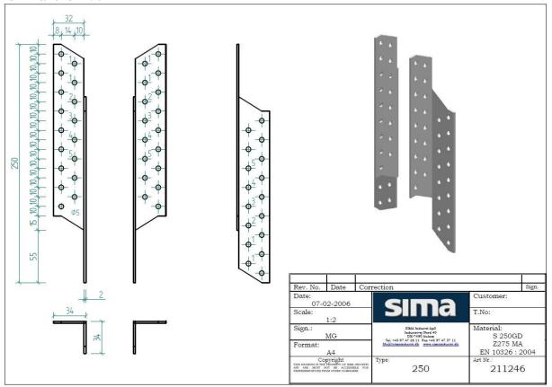
Additionally the bracket can be made from 1,5 mm pre-galvanized steel grades S350GD to Grade S500GD +  $\pm$  min. Z275 according to EN 10346 named Purlin Anchor 250PL
