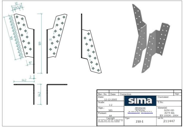
Additionally the bracket can be made from 1,5 mm pre-galvanized steel grades S350GD to Grade S500GD + min. Z275 according to EN 10346 named Purlin Anchor 210-1PL
