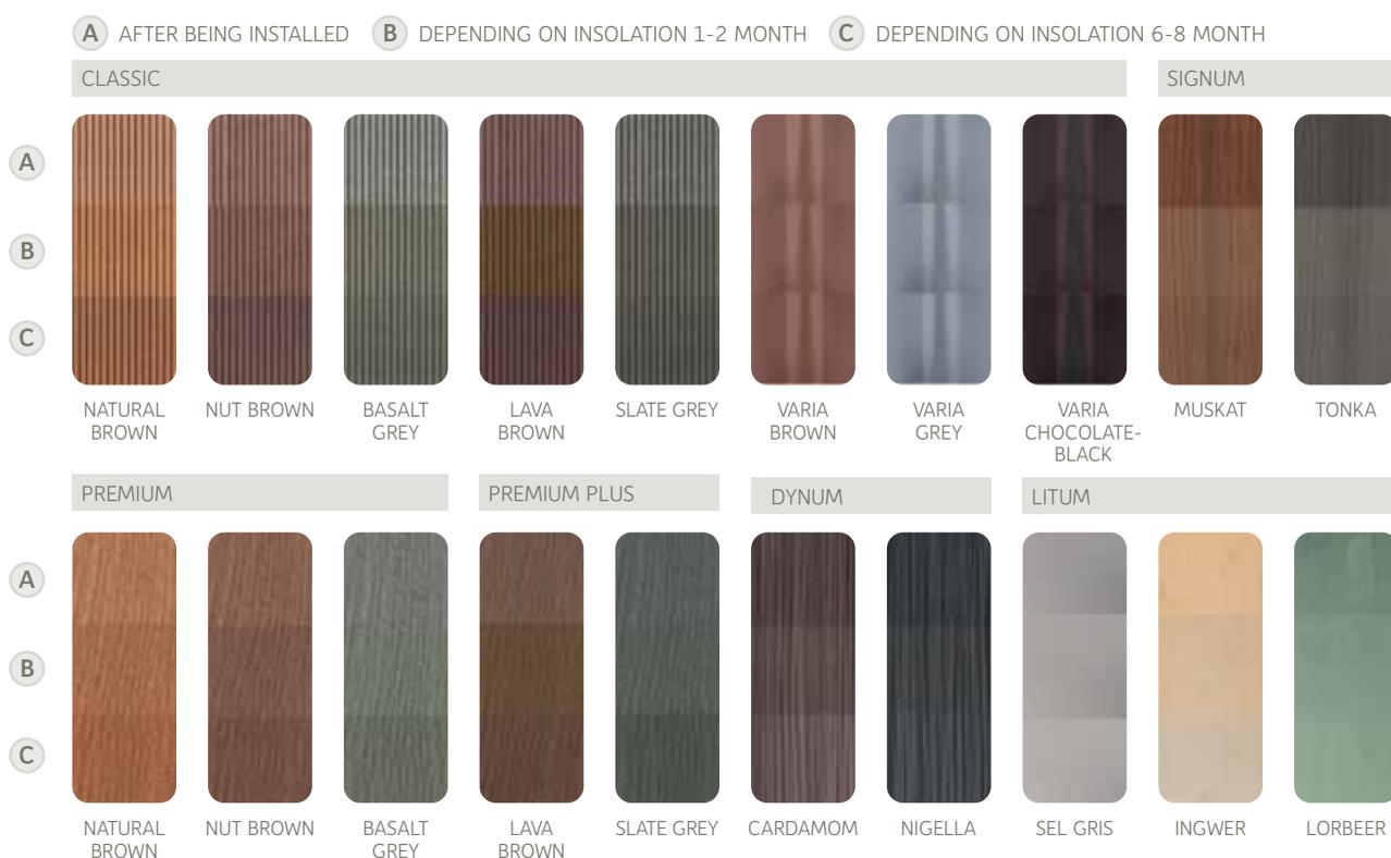
The natural colour maturation is checked with accelerated weathering test and instruments. Sunlight and humidity is simulated with periodic changes; 1000 hours of weathering correspond with approx. one year of outdoor exposure.
