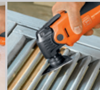
Flat slipeplate for smale mellomrom.
