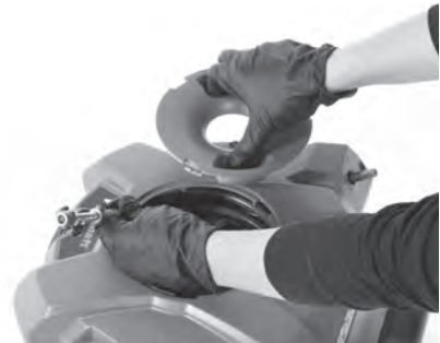
Figure 7B – Retrieve Chain Knocker/Cable
