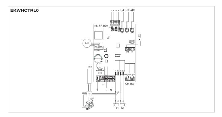
Rigid or flexible wires with a 0.2 to 1.5 mm² cross-section (0.75 mm² if two wires are connected to the same terminal block) can be inserted in the 4 spring-loaded terminal blocks (ref. A) for connection of the wall-mounted controller EKWHCTRL1. If the wires have wire end ferrules with a plastic collar, the maximum cross-section is 0.75 mm².
