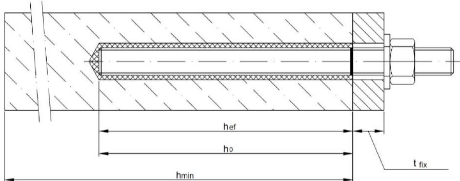
**Installation reinforcing bar Ø8 up to Ø32**
