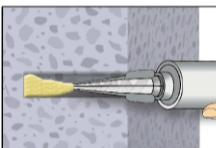
6. Starting from the bottom or back of the cleaned anchor hole, fill the hole up to approximately two-thirds with adhesive. Slowly withdraw the static mixing nozzle as the hole fills to avoid creating air pockets. For embedment larger than 190 mm an extension nozzle shall be used. Observe the gel-/ working times given in Table B5 or B6.
