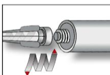
3. Attach the supplied static-mixing nozzle to the cartridge and load the cartridge into the correct dispensing tool. Cut off the foil tube clip before use. For every working interruption longer than the recommended working time (Table B5 or B6) as well as for new cartridges, a new static-mixer shall be used.
