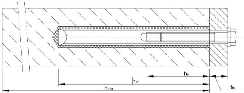
$t_{fix}$  = thickness of fixture
