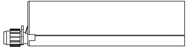
**Two part foil in a single piston component cartridge**
