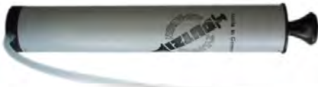
MAC - Hand pump (volume 750 ml) Drill bit diameter ( d_0 ): 10 mm to 20 mm Drill hole depth ( h_0 ): < 10 d_{nom} Only in non-cracked concrete
